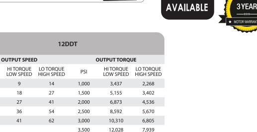
Output speed and torque specifications are THEORETICAL. Speed and torque output are dependent on the overall system efficiencies associated with the prime movers hydraulic system. This document should be used for information and comparative purposes only. When determining criteria, & application specific information is required, please contact DIGGA.
