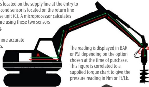
The reading is displayed in BAR or PSI depending on the option chosen at the time of purchase. This figure is correlated to a supplied torque chart to give the pressure reading in Nm or Ft/Lb.
